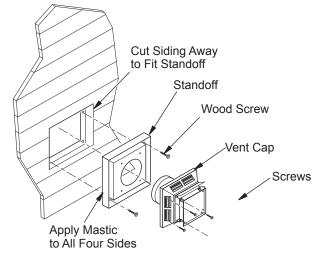
Figure 11 - Installing Siding Standoff (Combustible Exterior Wall)
